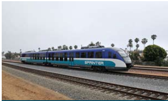
Left: Sprinter's sleek profile. Because the Sprinter's DMU cars are bidirectional, there is no need for looping at the end of the route. Right: The Sprinter arriving at one of its stations.
