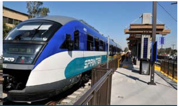
Left: Sprinter's sleek profile. Because the Sprinter's DMU cars are bidirectional, there is no need for looping at the end of the route. Right: The Sprinter arriving at one of its stations.
